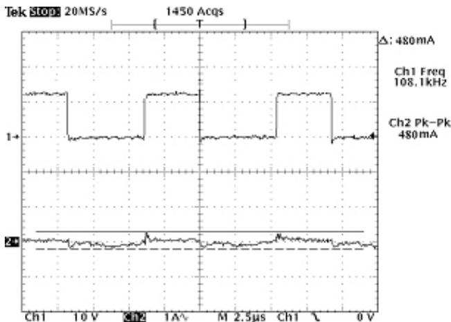
Figure 6b. Operating Ripple Current with L2
