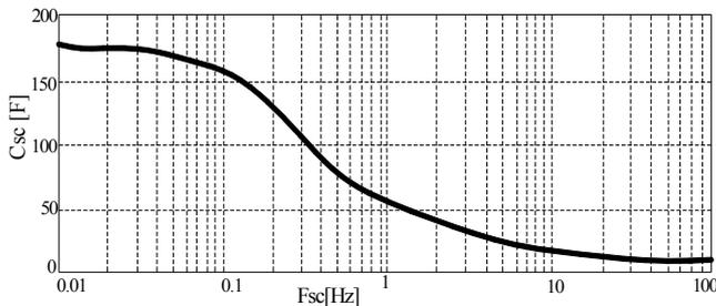
Figure 1b. Capacitance vs. frequency plot of Ultra-capacitor
