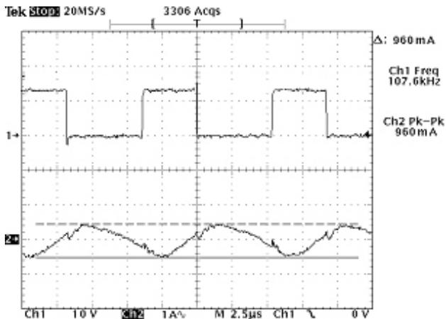
Figure 6a. Operating Ripple Current without L2
