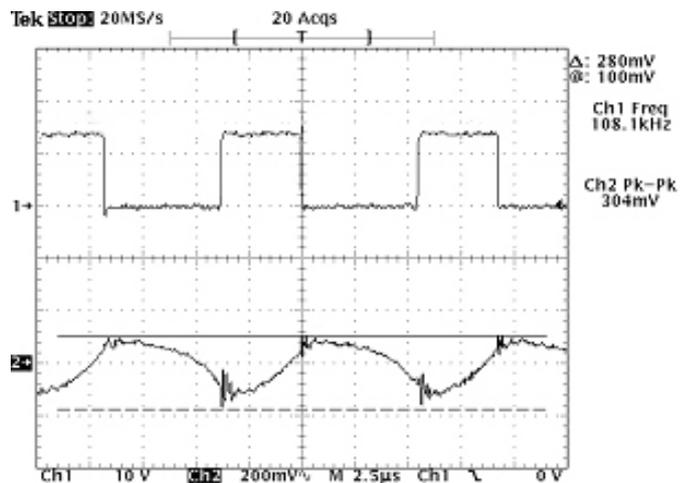
Figure 5b. Operating Ripple Voltage with L2
