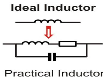
Figure 2. Interwinding Inductor Capacitance
