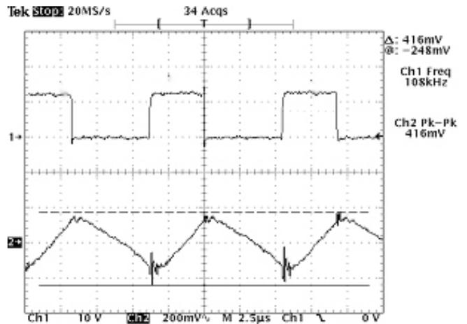
Figure 5a. Operating Ripple Voltage without L2
