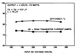
Fig. 13. Performance of combination series-parallel converter bread-
