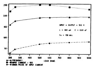
Fig. 9. Characteristics of parallel-resonant converter.
