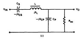
Fig. 4. AC equivalent circuits for resonant converters. (a) Series loaded. (b) Parallel loaded. (c) Series-parallel loaded.
