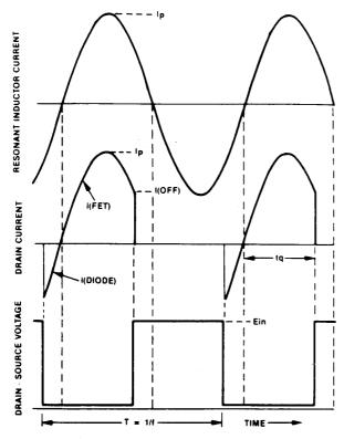
Fig. 2. Ideal resonant converter waveforms
