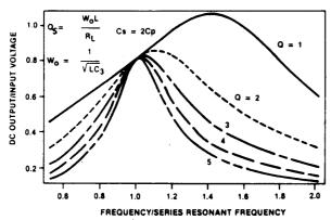
Fig. 8. Combination series-parallel converter gain (valid for frequencies at or above resonant peaks only).
