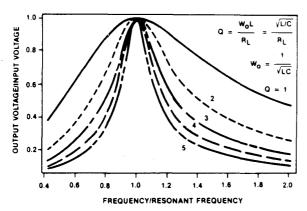
Fig. 5. Series-resonant converter gain (valid for frequencies at or above resonance only).
