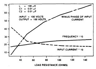
Fig. 10. Characteristics of combination series-parallel converter.
