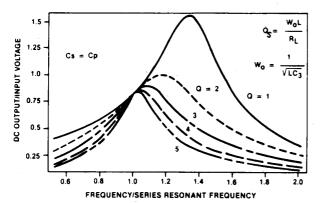
Fig. 7. Combination series-parallel converter gain (valid for frequencies at or above resonant peaks only).
