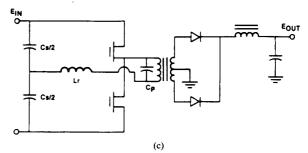
Fig. 1. Three types of half-bridge resonant converters. (a) Series loaded. (b) Parallel loaded. (c) Series-parallel loaded.
