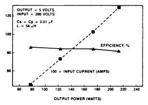
Fig. 12. Performance of combination series-parallel converter breadboard.
