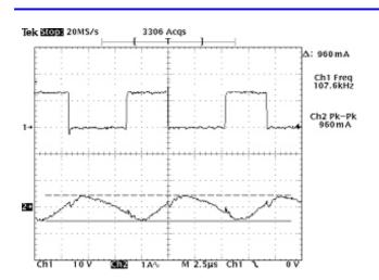
Figure 6a. Operating Ripple Current without L2
