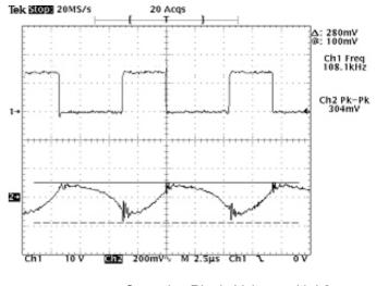
Figure 5b. Operating Ripple Voltage with L2
