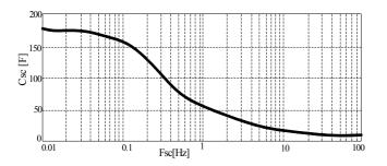
Figure 1b. Capacitance vs. frequencyplot of Ultracapacitor
