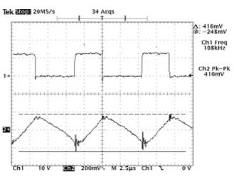
Figure 5a. Operating Ripple Voltage without L2
