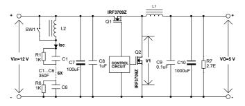
Figure 4. Buck converter circuit model with Ultra-Capacitor at the input.
